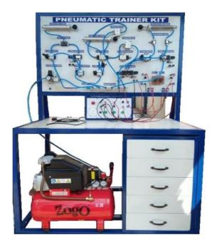
Electro Pneumatic Workbench is designed to understand fundamental of design, construction and application of Pneumatic components and circuits. We have two variants of Workbench one is without PLC and another is With PLC, user can select any according to hid application, todays industries are moving towards hybrid Industrial Automation systems with the help of PLC and other Pneumatic components and modules.
