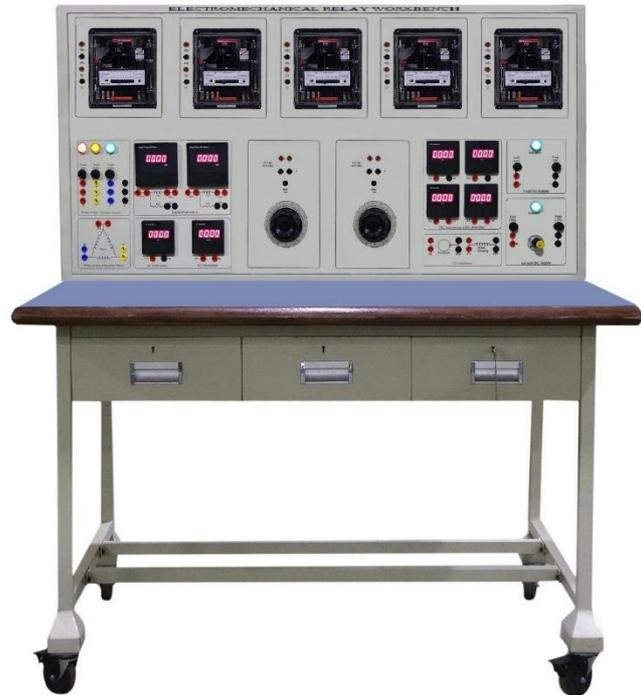
The Different Relay operates due to differential current flowing in the circuit. When current between two sections vary from a known and permissible value, the relay gets tripped and protects the connected device.
